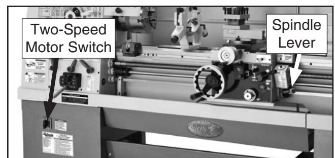
Figure 24. Location of the two-speed switch.
